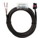
The cable is available in either 20', 40 or 60' lengths with a removable Packard connector to provide easy serviceability. The wire is sealed and crimped to the Packard connector providing a liquid tight environment and strain relief. Media compatibility: Refrigerants (freons) and ammonia.
